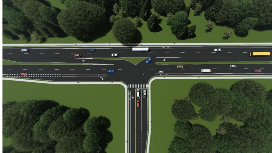
Photo 6: Unsignalized Continuous Green T-Intersection Example
